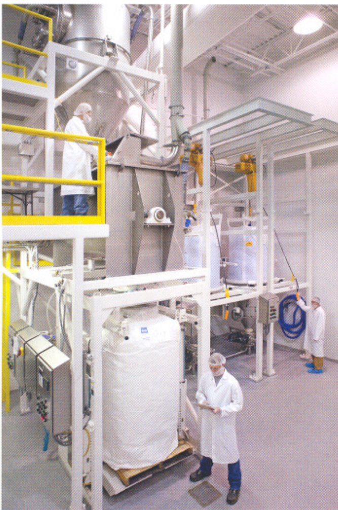
Overall view shows two bulk bag dischargers for whole wheat flour and nonfat dry milk, pneumatic conveying lines, weighing hopper, hand addition of ingredients, the ribbon blender, and final mix in the bulk bag below blender.
