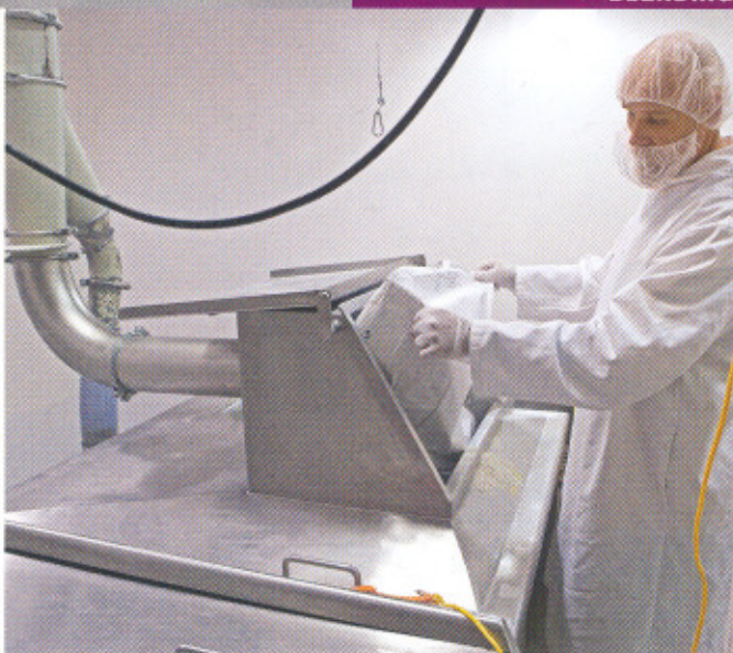
Small amounts of proprietary ingredients are added to the blender by hand.
