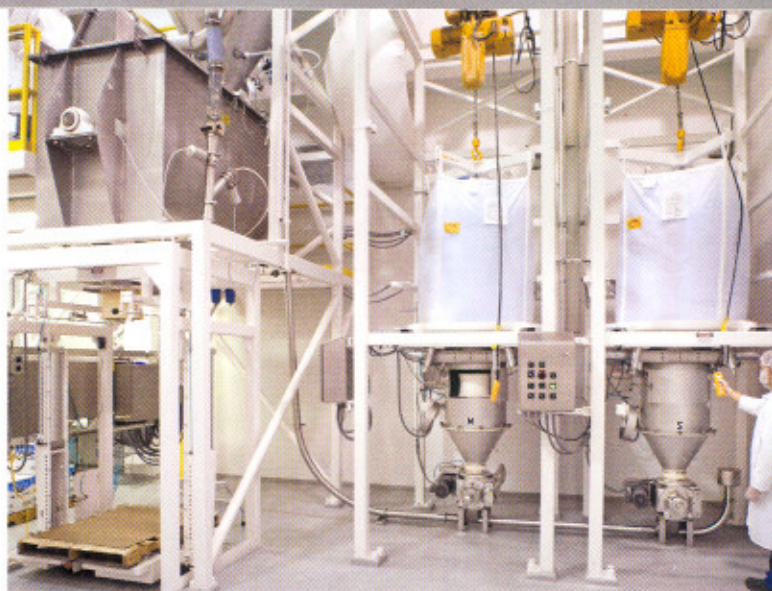
From each bulk bag, dry whole wheat flour and instant nonfat dry milk are pneumatically conveyed to a weighing hopper and then into the Munson HD-3-1/2-7 SSD Double Ribbon Blender.
