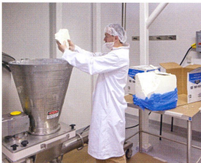
Shortening is added to blender, equipped with a shortening extrusion system, by means of a progressive cavity pump.
