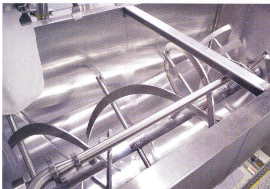
Designed for thorough mixing, easy cleaning: Tight tolerances between ribbon blades and blender trough minimise residual material remaining in the vessel after discharge. Agitator length-to-width ratio of 2-to-1 yields uniform blends in minimum cycle times. A spray line is included for liquid additions.
